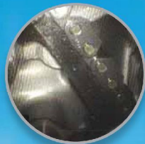
Timing chain in Honda 500 cc motorcycle
