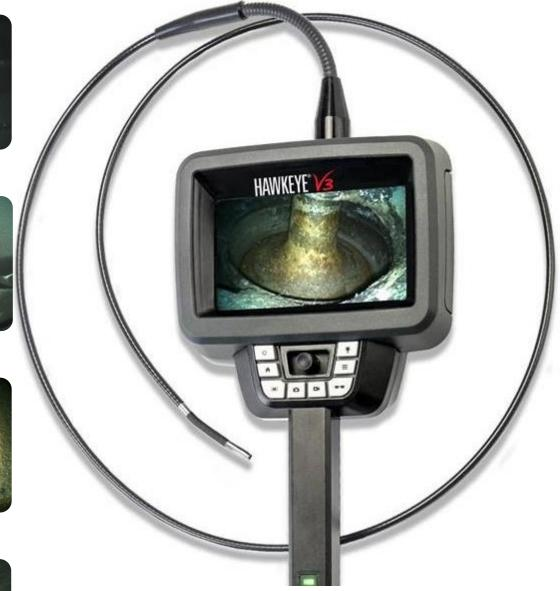
The Hawkeye<sup>®</sup> V3 *HD* Video Borescope features a new Micro *HD* video camera, and custom-engineered image processor. The 4and 6-mm Hawkeye V3's deliver simply the best image quality of any borescope on the market today! Video footage, and still images, captured by the V3 appear crystal clear and with vibrant, lifelike colors.
