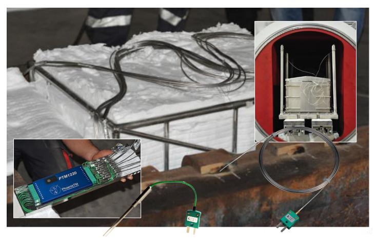
All PhoenixTM thermocouples are manufactured to the highest quality standards and conform to the ANSI MC96.1 special limits specification or IEC 60584 class 1. The thermocouple construction is designed to withstand rough handling, and the insulation material and plug terminations are colour coded to conform to IEC 60584. For high temperature applications (up to 1300°C) PhoenixTM supply a range of sheathed, mineral insulated, thermocouples terminated with a high temperature plug.
